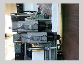
Spindle No. 2 Ø5 drill bit as standard (can be equipped with cutter up to Ø45)
