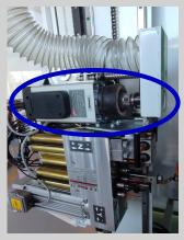
High frequency motor, 18000rpm, 3 hp, to make routing, milling, cuts, slots, decorative design, corners retails, Gola arcs, and more. It replace the saw unit to make the groove, because is faster, only one pass to finish the width of the groove using the right tool
